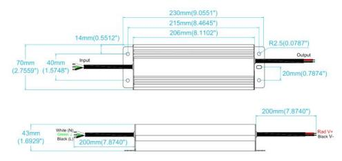
1. The input terminal has a 3-pin wire, of which the green wire is to be connected to the ground, black and white connected to AC L and N.
