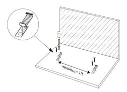
**Step 5** Gently push the neon into the mounting clips from one direction with palm instead of finger.
