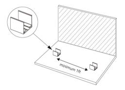
**Step 5** Gently push the neon into the mounting clips from one direction with palm instead of finger.
