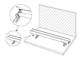
**Step 6** Plug in power after installation, make sure the neon flex is correctly lit up. Adjust to the adjustable clip to a desired angle.
