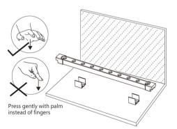
**Step 2** Determine the desired location and lengths of neon to be installed. Leave enough distance for power cable to reach the power supplies.
