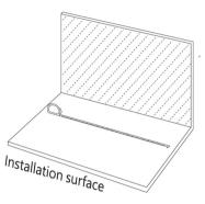
**Step 4** Install the mounting clips into position with screws. Make sure the head is flush or lower the base of the channels. DO NOT screw at an angle.
