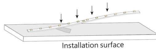
**Step 3** Gently press the LED strip back and forth to make sure that it's flat and firm without any air pockets.
