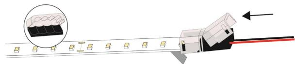
**Step 4** Make sure that both covers of the strip to cable connector are firmly locked.
