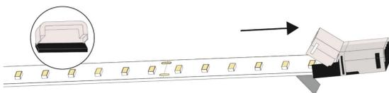
**Step 1** Peel off a small section of 3M tape on the back of the LED strip to install connector.
