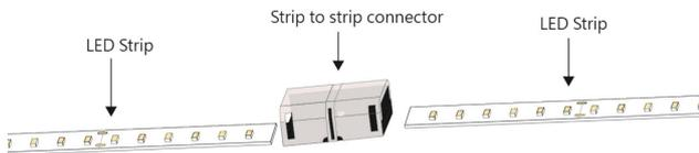
**Step 2** Open the cover of the strip to strip connector. Put the LED strip directly onto the connector. Close the cover till it's locked in.
