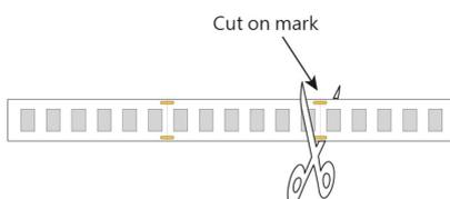
**Step 2** Use factory-recommended cutter, gently cut straight down through the body of the product directly on the cutting increment mark. DO NOT cut diagonally or horizontally as this may damage the product.
