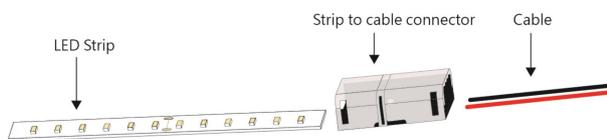
**Step 2** Open the cover of the strip to cable connector. Put the LED strip directly onto the connector. Close the cover till it's locked in.
