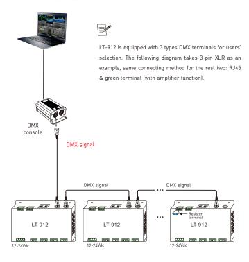
If the recoil effect occurs because of longer signal line or bad line quality, please try to connect 0.25W 90-120Ω terminal resistor at the end of each line.
