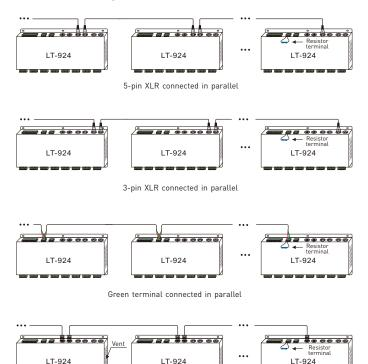
Rj45 connected in parallel
