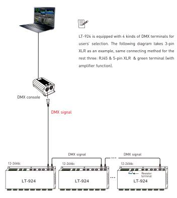
\* If the recoil effect occurs because of longer signal line or bad line quality, please try to connect 0.25W 90-1200 terminal resistor at the end of each line.
