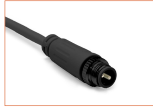
MCB-2P-67 Male connector, 11.81in. (300mm) black cable, 2 pin, IP67, Wet, 18 AWG
