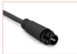
MCB-2P-67 Male connector, 11.8in. (300mm) black cable, 2 pin, IP67, Wet, 18 AWG
