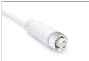
FCW-2P-67 Female connector, 11.8lin. (300mm) white cable, 2 pin, IP67, Wet, 18 AWG
