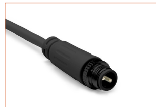
MCB-2P-67 Male connector, 11.8lin. (300mm) black cable, 2 pin, IP67, Wet, 18 AWG
