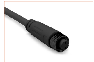
FCB-2P-67 Female connector, 0.98ft (30cm) black cable, 2 pin, IP67, Wet, 18 AWG
